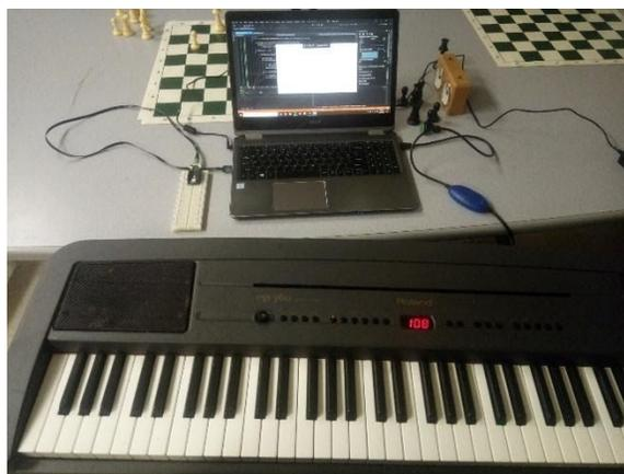
**Figure 4 - The keyboard sends signals to the computer using a M-audio Midisport Uno**
