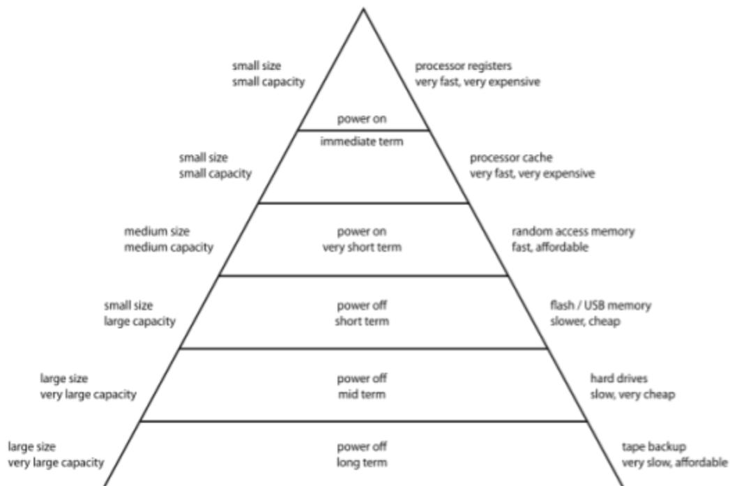
**Figure 1.** Shown is the hierarchy of computer memory in relation to size, speed, cost, and longevity. The fastest form of computer memory is the registers that reside on the processor chip while the slowest form are external drives. Registers are tiny and only hold information as long as power remains in the unit. External drives can store information indefinitely with or without power [5].
