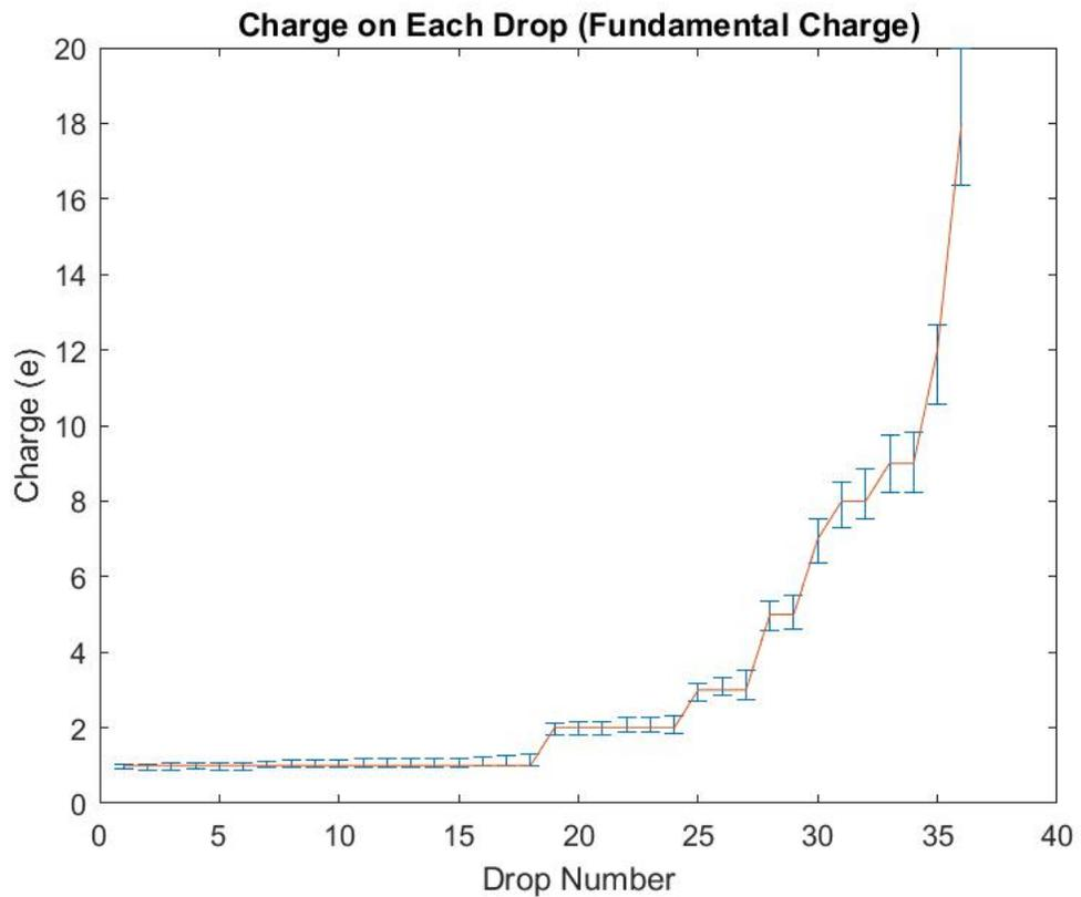
**Figure II:** Measured values of  $q$  in terms of the measured fundamental constant  $e$  for each drop sorted from smallest to largest, with error bars shown. Values of  $\frac{q}{e}$  were rounded to the nearest integer, and all were within the bounds of error.
