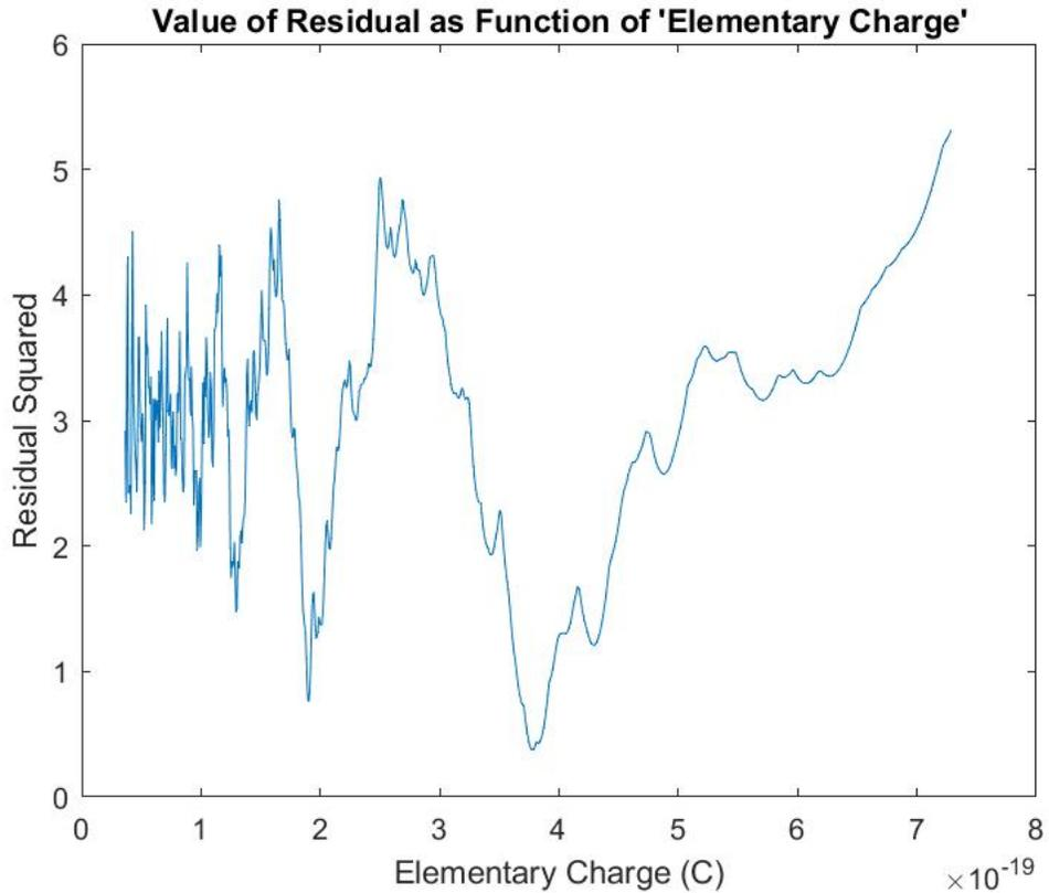
**Figure I:** Value of Residual Squared for Test Fundamental Charges Ranging From  $3.64 * 10^{-21}$  to  $6.86 * 10^{-18}$  Coulombs. Plot window reduced from full range tested for ease of viewing (see **Figure III** in the Appendix for full range).
