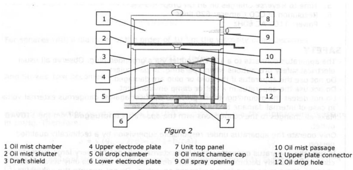
Figure 1: This image was taken from the United Scientific Supplies manual; it shows the various components of the oil drop apparatus.
