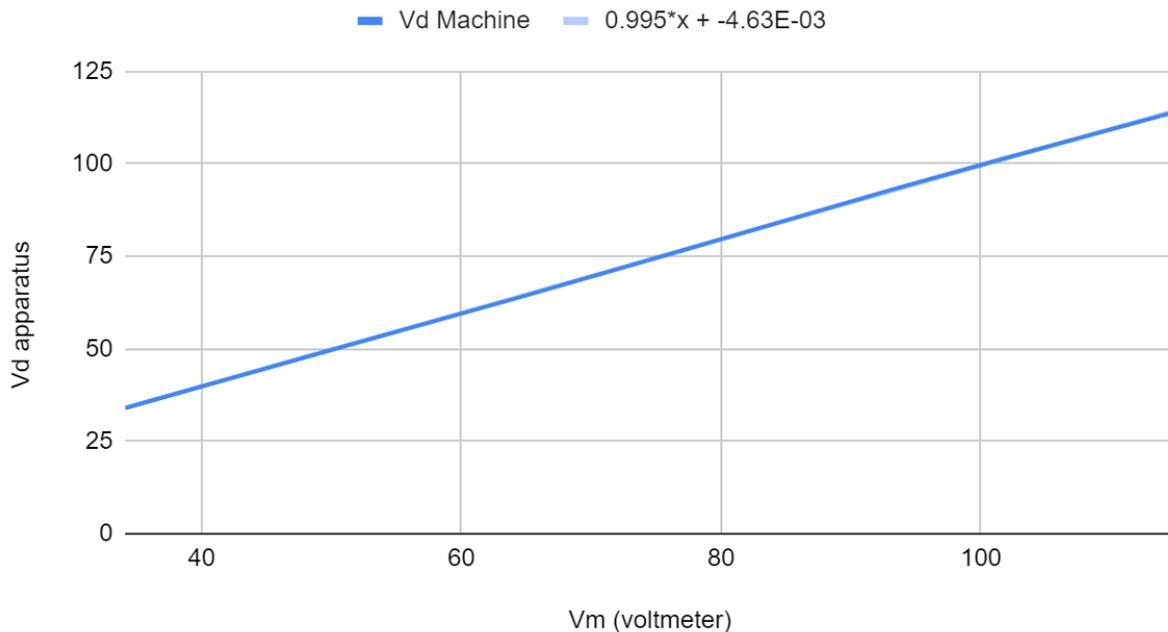
figure 2: This chart is for the calibration of the oil drop apparatus. Vd is the voltage read from the apparatus, while Vm is the voltage measured from a voltmeter. A linear line was used to find the relation between the two. Both axis are measured in volts.
