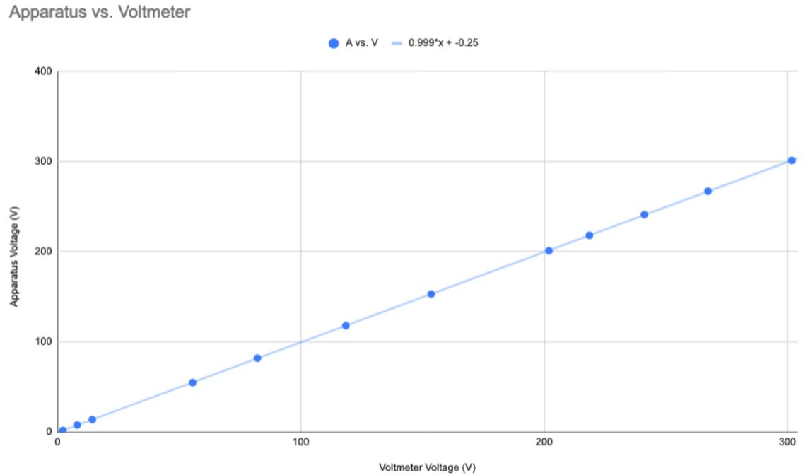
Figure 3: Plot of the voltage displayed on the apparatus vs. that on the voltmeter. The equation of the best fit line is shown above the plot, from which the slope is used to correct subsequent voltage readings from the apparatus.
