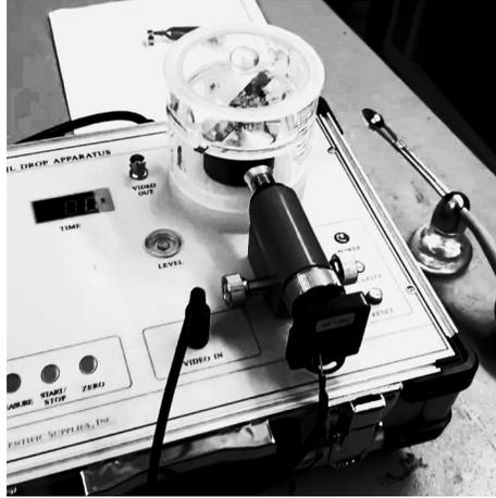
Figure 2: Image of a section of the MODA01 apparatus with the oil drop device above it. The camera is the dark device inserted into the draft shield of the oil drop device.
